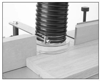
Figure 19. Safety guard adjusted properly.
